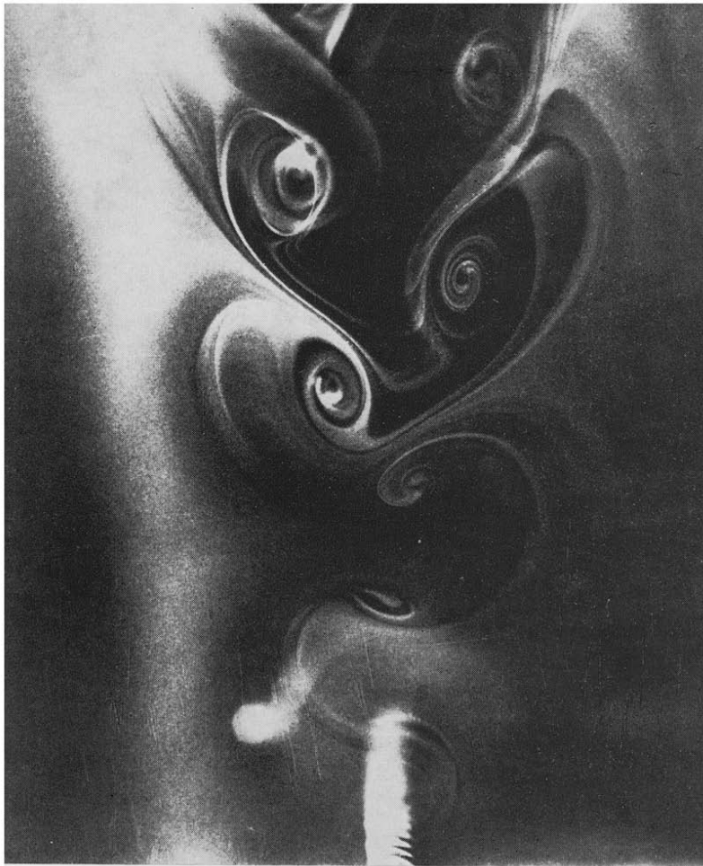
FIG. 3. Flow visualization of vortex shedding from a vibrating six-stranded cable. The Reynolds number based on cable outer diameter and free stream speed is 220. The vibration frequency is 110 per cent of the Strouhal frequency for this Reynolds number and the amplitude is 30 per cent of a diameter.
